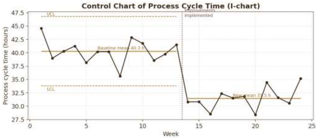
Figure 8. Control chart of process cycle time (I-chart).
